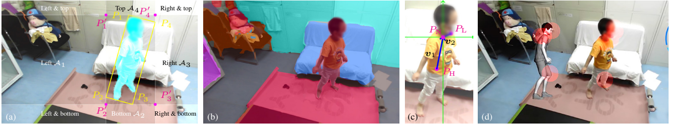
Fig. 6: Illustrations of (a) sub-space division, (b) scene segmentation, (c) key points and local coordinate system, and (d) the rendered AR effect.
